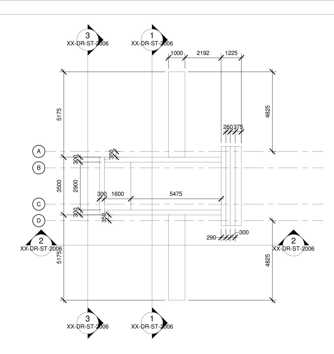
Plan View on Abutment 1 Scale: 1:100
