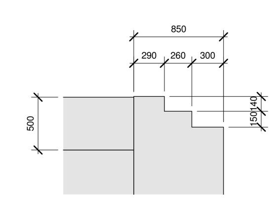
Abutment Detail (A) Scale: 1:25
