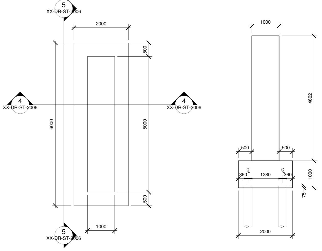
Plan View on Pier Scale: 1:50
